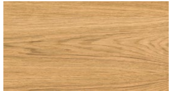
Crown cut structure
