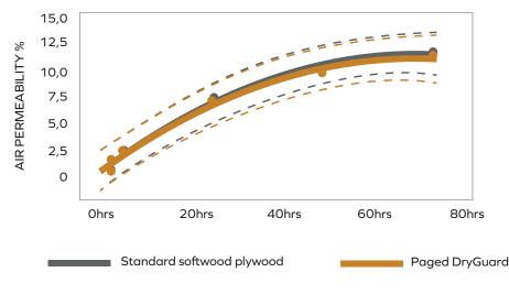
Laboratory tests according to internal Paged LabTech standard 17 S/2020: Air permeability.
